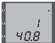
Fig. Operating hours meter of the measured value display The UMG 96RM shows the number 140.8 h in the operating hours meter. This corresponds to 140 hours and 80 industrial minutes. 100 industrial minutes correspond to 60 minutes. In this example, 80 industrial minutes therefore represent 48 minutes.
