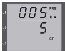
Fig. Current transformer programming mode The primary and secondary currents can be changed using buttons 1 and 2 (cf. page 40).
